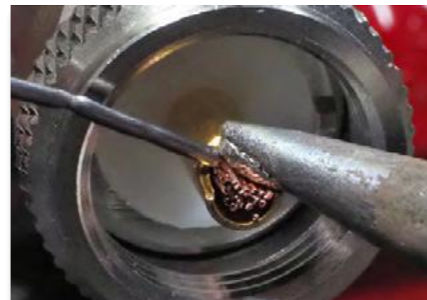
To fill the cavity of the "UHF" connectors repeat the welding in 2-3 times by adding tin every time.
