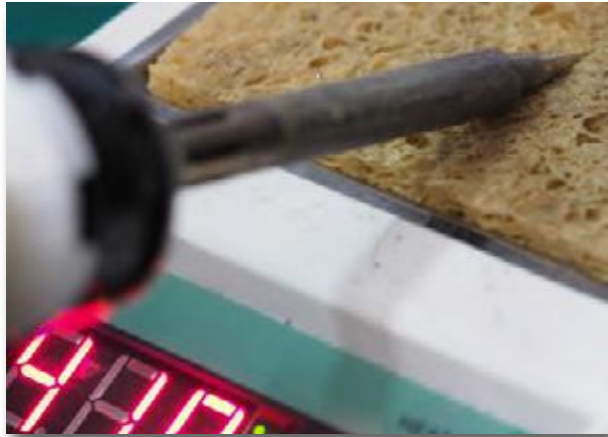
(1) Wipe the welder tip on a wet sponge.
